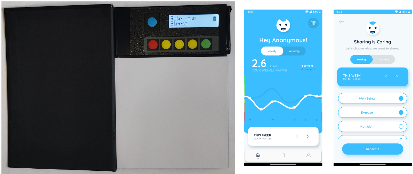
Fig. 3. A digitally augmented notebook (DAN) on the left with an LCD and a button to select a wellbeing aspect, and a group of five buttons to rate said measure. On the right, two of Danny's screens, including a visualizations page and a customizable sharing feature.
